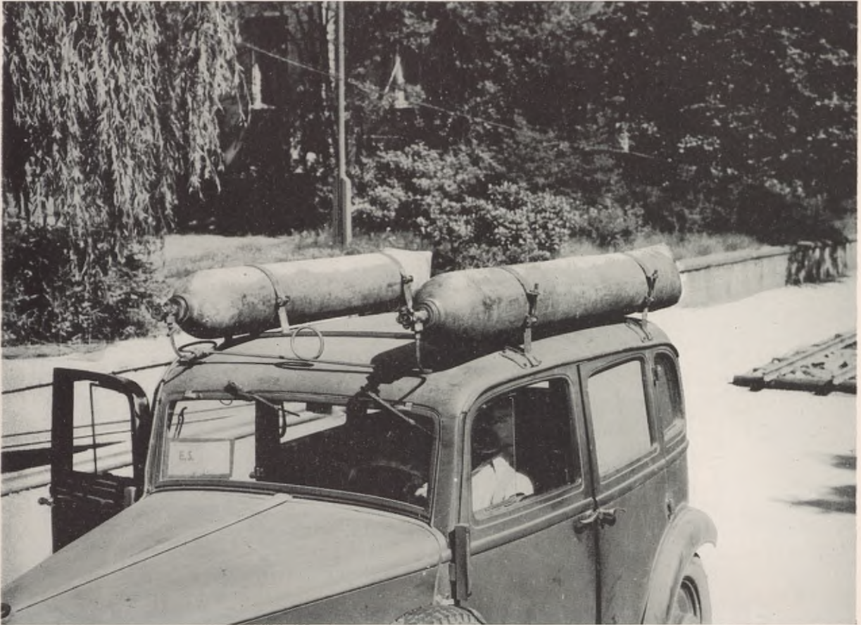
FIGURE 144. Compressed gas for auto fuel—typical installation. Gas obtained from sewage disposal plants and gas works.
