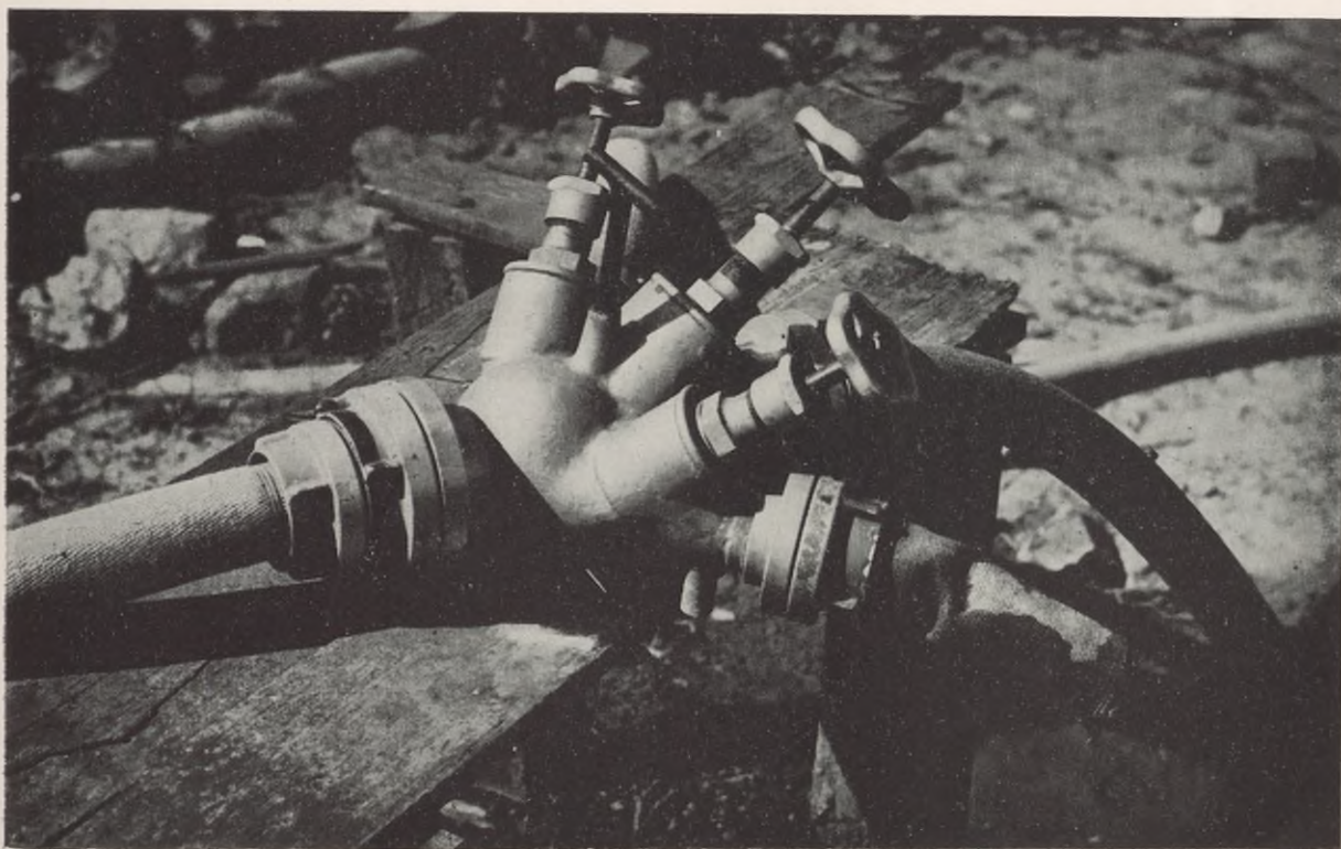
FIGURE 117. Multiple valved distributor hose used by water line wardens and repair teams following air raid.
